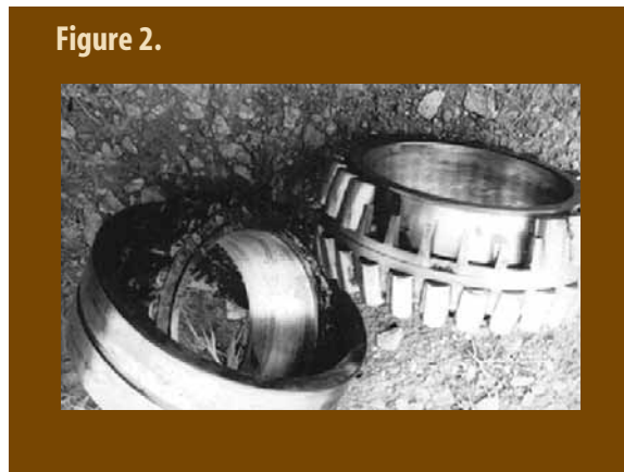
Failed rolling bearing.
