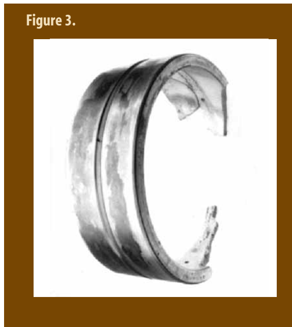
Broken outer ring of rolling bearing.
